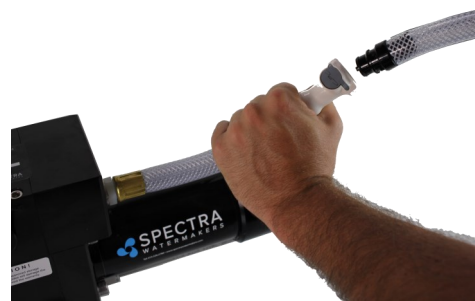
Feed pump module valves in FLUSH position:
