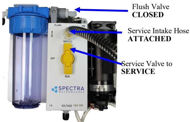
Valves in SERVICE position:
