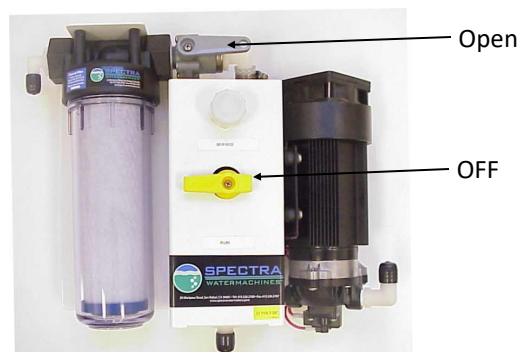
Feed Pump Module A with valves in the FLUSH Position:
